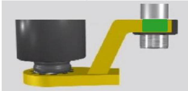
Figure 4.2.4-1: Correct Reaction Point
